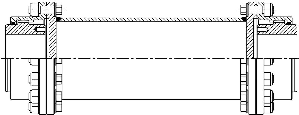
A tubular fabricated spool spacer is used as a center section between flex half couplings that are mounted on the shaft ends that are being joined together. The flex half couplings can use standard hubs, reversed hubs, extended hubs, or mill motor hubs.
