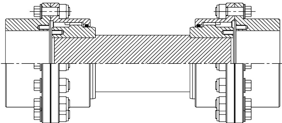
In this design rigid hubs are mounted on the shaft ends that are being joined together. The floating shaft center section consists of a machined shaft with flex halves on both ends. The flex half couplings can have standard hubs, reversed hubs, or extended hubs.
